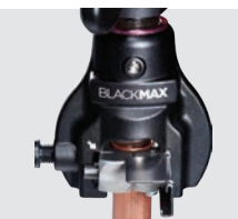
Eccentric forming cone for easier flaring
