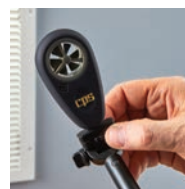
Thumbwheel for attaching/removing threaded universal end
